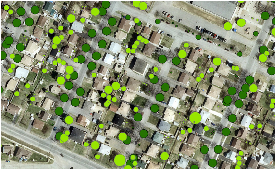
Figure 3 A screen capture from ArcGIS® displaying the public (dark green) and private (light green) trees after the buffers had been applied, to produce a realistic representation of canopy cover based on each tree's crown width class
